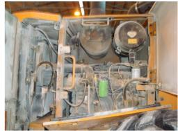
Engine Bay coated inside after 2yrs- 1 recoat. Dust but no rust!!
